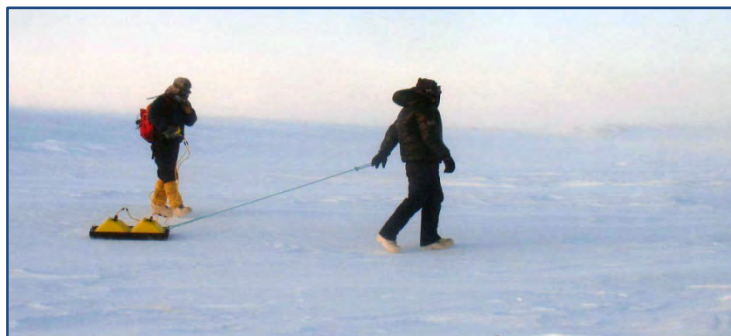
Figure 2 Collecting ground penetrating radar data at a Fish Creek study lake.
